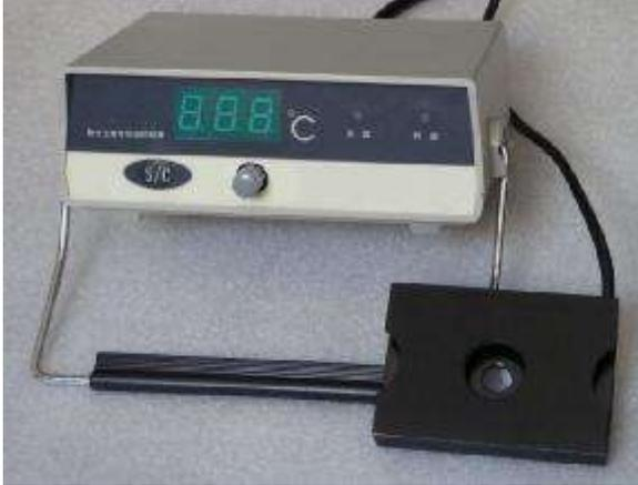
**Sperm microscope melting point heating stage
